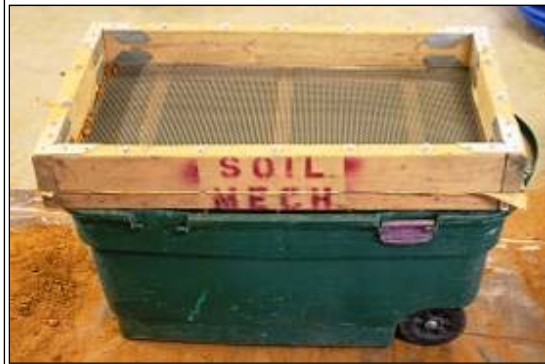
(c) Portable Bin and 4.75 mm Sieve
