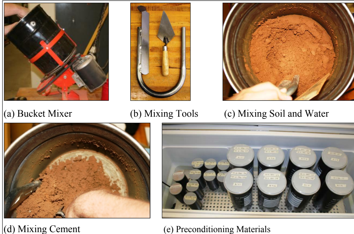
Figure 4.12 Mixing Equipment, Mixing Operations, and Material Conditioning
