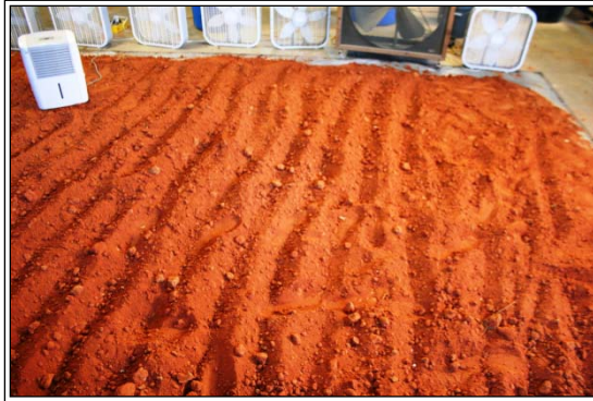
(a) Air Drying of Soil
