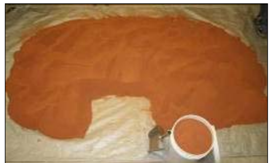
(h) Placing Soil into Buckets
