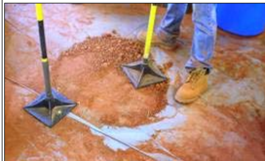
(e) Tamping of Plus 4.75 mm Material
